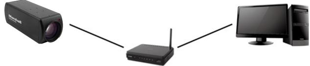
2. If the camera is connected to the computer directly, the computer IP address must be modified to have the same network segment as the camera
